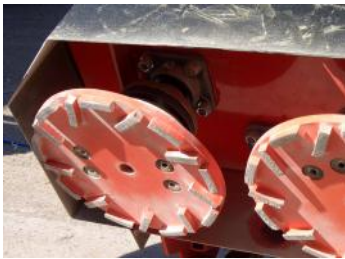
Machine fitted with 250mm diamond discs
