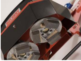
Machine fitted with carborundum blocks
