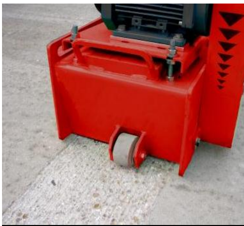
Cleaning & keying concrete
